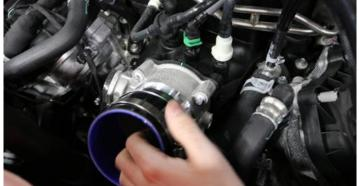
9. Locate the Ø3.5" straight sleeve and two #56 clamps. Install straight sleeve with one clamp onto throttle body and tighten clamp with flathead screwdriver or ratchet and 8mm socket. Loosely place the other clamp onto straight sleeve.
