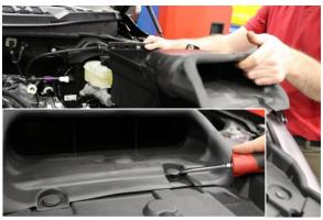
**8.** Remove the two factory scoop retaining clips using a trim removal tool. Remove air box and scoop from vehicle.
