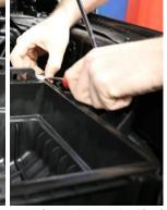
Disconnect wiring harness from lower half of factory air box by using a trim removal tool on the wire clips.
