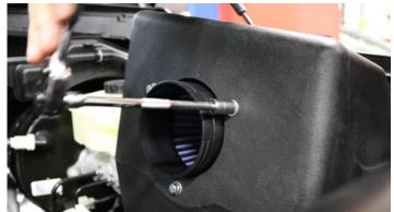
8. Locate three 6mm x 16mm bolts, three remaining .25" x .63" flat washers, and three remaining .25" lock washers. Attach filter adapter to air box and tighten using a ratchet and 10mm socket.
