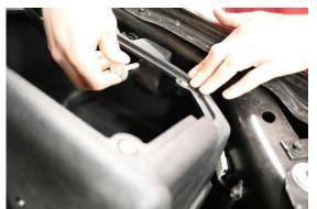
**5.** Locate the bolt from removal step 7 and attach the CORSA air box to the inner fender using a ratchet and 13mm socket.
