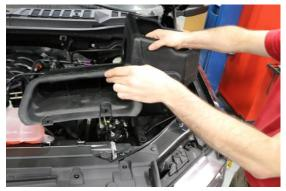
Install CORSA air box with scoop into the vehicle by inserting posts on bottom of CORSA air box into factory grommets.
