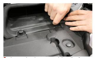
**6.** Locate the air scoop retaining clips from removal step 8 and attach factory scoop.
