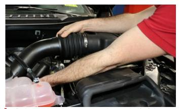
4. Release the clips securing the top half of the factory air box to the lower half and remove the duct and top half from vehicle.
