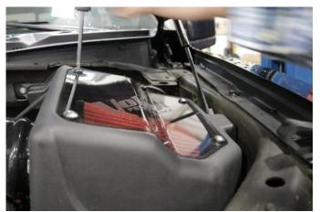
**13.** Locate the CORSA lid assembly, lid screws, and rubber washers. Install lid assembly onto air box using a Philips head screwdriver.
