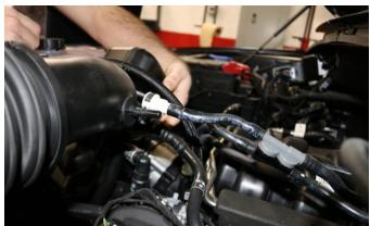
Disconnect vent connection from rear of factory air duct.
