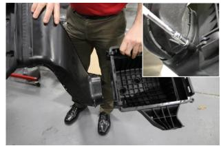
Remove bolt securing scoop to air box using a ratchet and 8mm socket. Separate scoop from air box.
