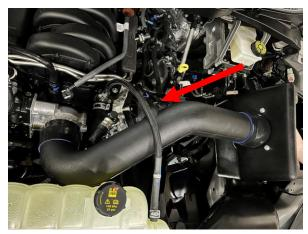
12. Connect vent line to fitting in air duct.
