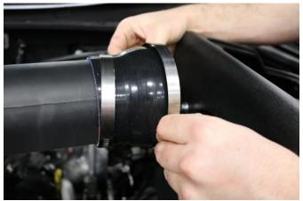
10. Locate CORSA air duct, threaded fitting, silicone reducer, remaining #56 clamp, and #64 clamp. Install fitting into threaded hole in duct, tighten with 13/16" wrench. Place smaller end of reducer approximately one inch onto air duct along with the # 56 clamp. Loosely place #64 onto larger end of reducer.
