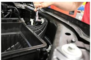
Remove the bolt securing the factory air box to the inner fender using a ratchet and 13mm socket.
