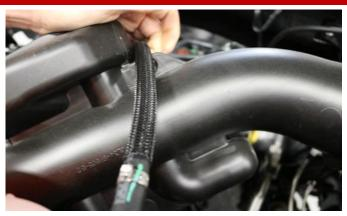
**2.** Pull the coolant hose from retaining feature on factory air duct.
