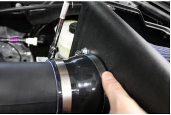
11. Install air duct into vehicle by placing the reducer onto the filter adapter and the opposite end into the straight sleeve clamped to the throttle body. Adjust duct as necessary and tighten all clamps using a flathead screwdriver or ratchet and 8mm socket.
