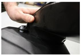
3. Locate the factory scoop, the 6mm x 25mm bolt, one .25" x .63" flat washer, the .25" x .75" flat washer, one .25" lock washer, the .25" spacer, and the 6mm nut. Attach air scoop to air box placing the spacer between the scoop tab and air box. Tighten hardware with 10mm wrenches.
