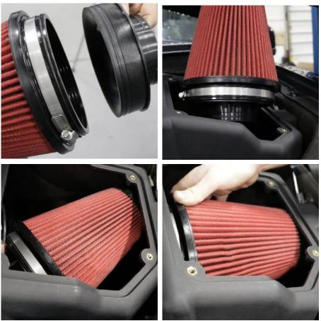
1. Locate filter and filter adapter and insert the filter adapter into filter. Tighten clamp enough that it won't fall off filter but leave loose enough to rotate. Insert the filter into the air box with the adapter side down. Rotate the top of the filter down into the air box and rotate the filter around and push the adapter through air box.
