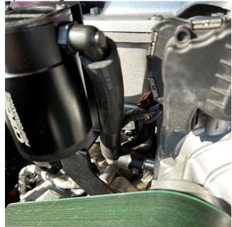
4. Install Hose B to the "B" side of the catch can and route the hose to the silver engine fitting located behind the bracket. Make sure both quick disconnect fittings click into place over the engine fittings (colors of fittings may vary).
