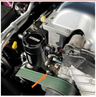
Using the 2.5mm Allen Wrench and 3 screws, attach the catch can to the bracket. Use the 2 flange nuts and an 15mm wrench to sandwich the bracket in between on the engine bolt.
