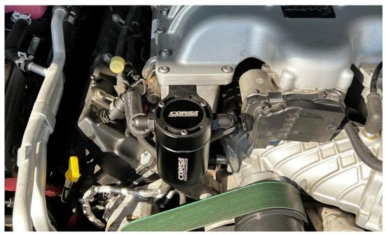
**5.** Make sure all fittings are secured in place and hose is pushed all the way over the barbed ends of the fittings. Reinstall engine cover.
