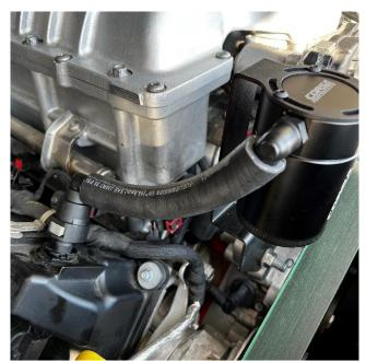
**3.** Attach quick disconnect elbow fitting to the ends of each hose. Install Hose A on the "A" side of the catch can and route the hose to the engine fitting to the left of the supercharger.
