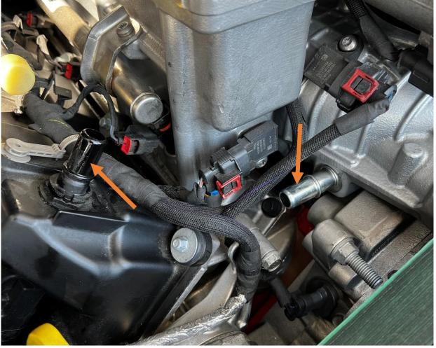
Remove passenger side engine cover by releasing it from the press fit tabs. Locate the PCV line on the passenger side of the engine and remove by pressing the tabs on the quick disconnect fittings.
