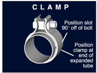
Using an air impact gun will damage the clamp and reduce its ability to effectively seal the joint. It may also cause the joint to separate, thereby causing damage to your exhaust system and to your vehicle.
