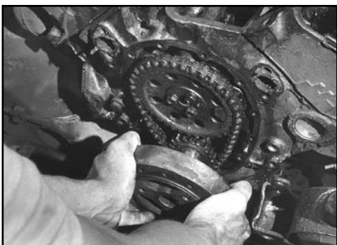
Figure 1. Turn the engine over by hand to align timing marks. Check a shop manual for exact alignment.
