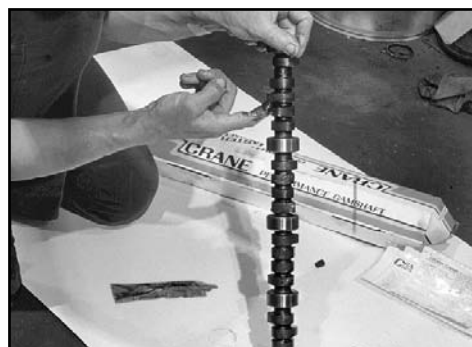
Figure 3. Apply lots of assembly lube to each cam lobe as shown.
