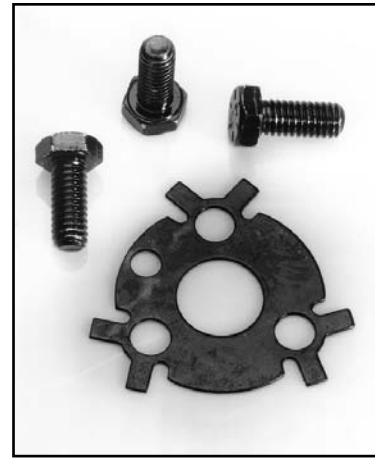
Figure 7. Crane Cams offers this unique camshaft locking plate and bolt kit for both small and big block Chevy's. It has tabs that can be bent over to prevent cam bolts from working loose. Good "insurance".
