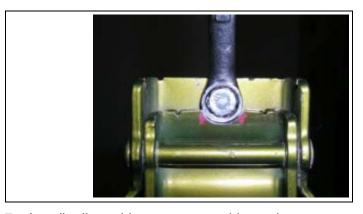
7. Install tailgate hinges, spacers, hinge plate spacers and hinge plate to jeep body. Make sure rounded edges of hinge spacer blocks are toward body.
