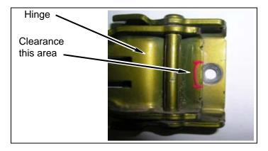
Mark and grind out area shown on factory tailgate hinges to allow clearance for *kit* **bolt** (8mm & tapered washer) and wrench during install.
