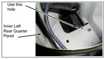
d. Align foot of bracket to location shown here and install *kit* **bolt** (1/4" x 1") with **hardware**.
