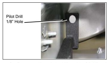
f. From top enlarge hole drilling with 3/8" drill and install *kit* **bolt** (3/8" x 1") and **hardware**.
