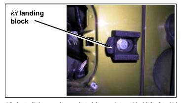
12. Install tire carrier rack to hinge plate with *kit* **bolts** (1/2" x 5-1/2") with **hardware** (1/2" brass washer, 1/2"
