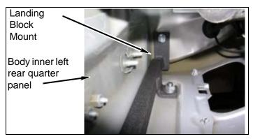
c. Insert kit landing block mount bracket under left rear of body and align holes in bracket to holes drilled. Make sure bracket is snug to inner body corner. Install kit bolts (5/16" x 3/4") and washers into bracket and snug but do not tighten.
