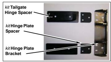
a. On inner two holes of hinge, Install using *kit* **bolts** (8mm-1.25 x 50mm) with **taper washers** (8mm). Do not tighten at this time.
