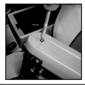
3. Place Arm Rest over console lid being careful not to scratch plastic cover. Place black plastic spacers between arm rest and console as shown. Secure with supplied phillips head screws.
