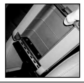
2. With console lid removed unscrew the 4 side torx head screws using the same T20 torx driver.
