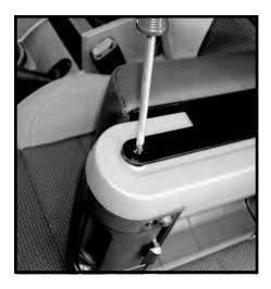
4. Place console lid and arm rest back onto lower console and secure using the 4 torx head screws saved from step 1.
