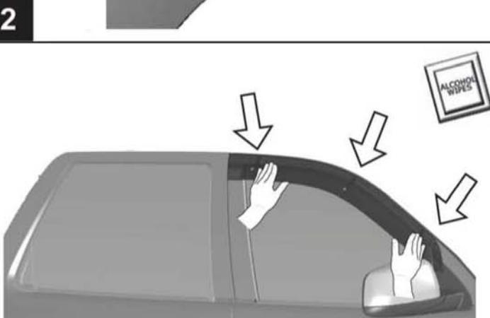
**Clean both inner and outer surfaces of door frame area with an alcohol pad, on front doors, be sure to also clean with alcohol pad the area of mirror support that deflector adhesive tape comes in contact with.**
