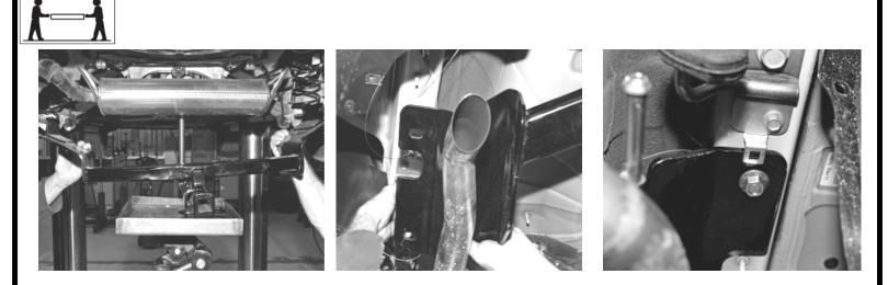
Lift trailer hitch into place while inserting fish wires through corresponding holes in trailer hitch. Insert drivers side first to position around muffler. Avoid the hanger tab. Remove the fish wires and hand tighten all the nuts.
