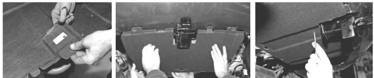
Trim center aero shield at marked lines. Re-install muffler isolators. Install clip nut from center hole on æro shield to front of hitch. Re-install center aero shield. Poke hole for center clip nut and reinstall fascia screws.
