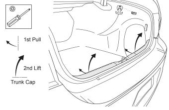
Open trunk, use torx T-25 wrench to remove bag hangers. Remove the inside trunk cap.
