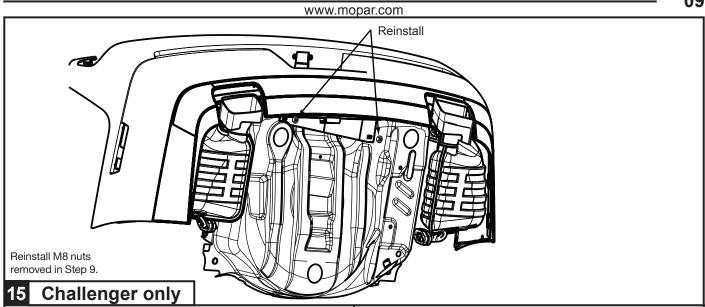
Reinstall and reconnect fascia and lights as necessary by reversing steps 2-4
