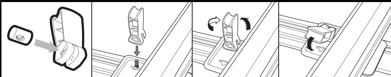
**a. Insert barrel nut into cam handle.**
