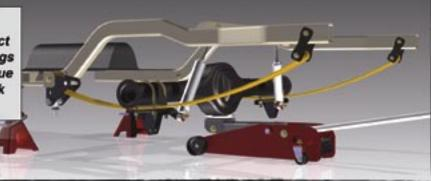
Compress the suspension before attaching transfer links. Apply grease or anti-cease to rod end threads. Thread both rod ends into link as illustrated. This will insure that rod ends thread out equally.
