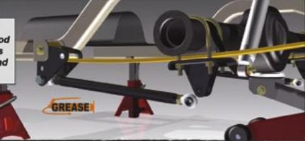
While holding the rear rod end by hand, begin to turn the link. Continue turning while applying foward pressure until rear rod end lines up with the lower mounting point. Tighten rear mount bolt and set a slight air gap between roll pin and springs upper surface.
