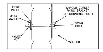
**9.** Fix the fans(s) to the radiator/condenser using the long bolts and nuts provided, together with the fibre and steel washers as per above diagram.
