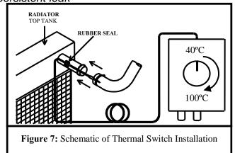
4. The EBP<sup>®</sup>23 has a built-in wiring loom with a female plug. You may wish to purchase the equivalent male plug to suit or you can dispose of this plug and crimp spade terminals on each end. Connect spade terminals to each pin of Thermatic switch. Refer to the #0401 Installation Instructions to ensure the EBP<sup>®</sup>23 is installed correctly
