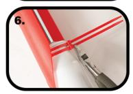
Position zip ties toward the top of the shock tube and firmly tighten your zip ties into place. You may cut the excess zip tie with a pair of cutters.
