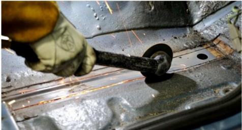
Figure 16 - Cut-Out Floor Section
