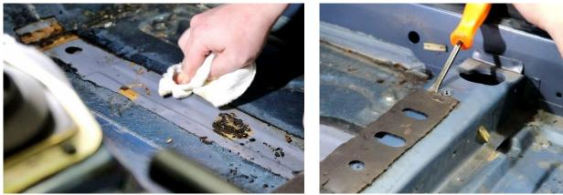
Figure 6 – Clean Cut Area and Remove Foam
