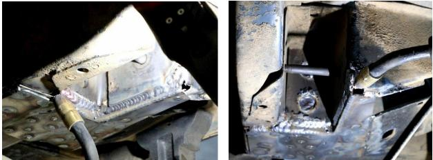
Figure 52 – Weld Link Pocket
