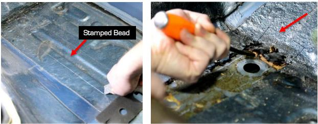
Figure 4 – Remove Floor Board Material
