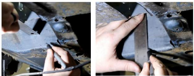
Figure 27 – Locate Torque Box Cut Lines
