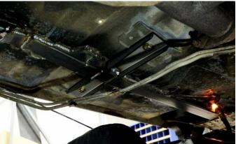
Figure 58 – Finish Weld Rear Connector
