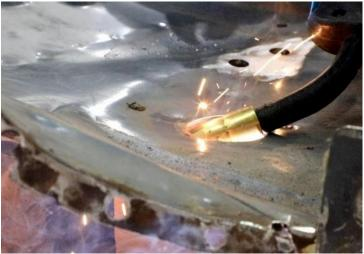
Figure 48 - Tack Weld Torque Box
