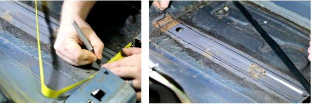
Figure 14 – Mark Inboard Cut Line
