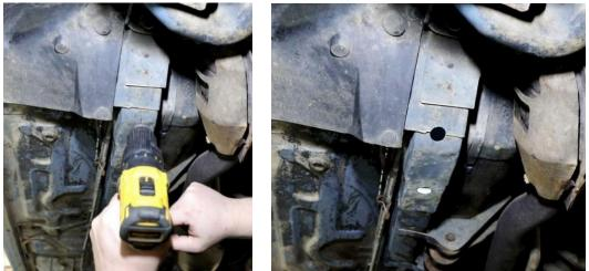
Figure 33 - Drill Plug Weld Location
