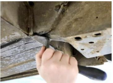
Figure 3 - Remove Brake Line Bracket
