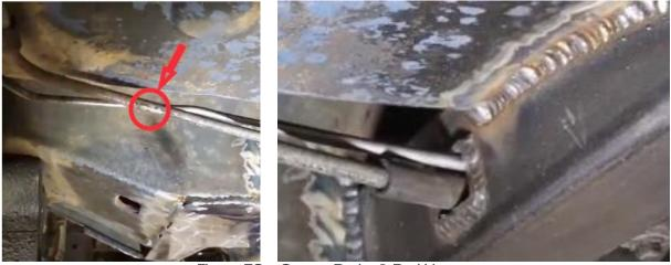
Figure 59 – Secure Brake & Fuel Lines
