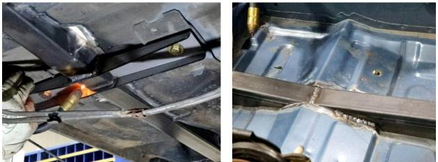
Figure 55 – Weld Seat Mount
