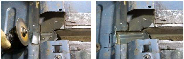
Figure 19 - Remove Floor under Seat Riser
