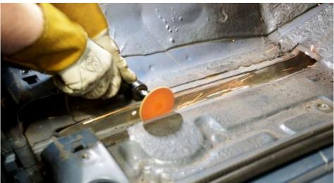
Figure 18 – Grind Cut Lines Page 8 of 23
