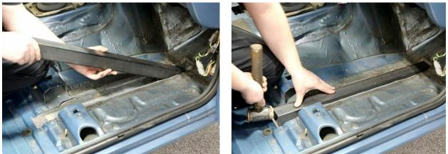
Figure 22 - Install Front Subframe Connector Assembly
