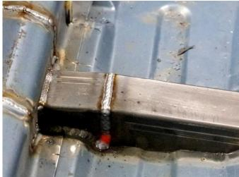
Figure 57 – Weld Front & Rear Connector
