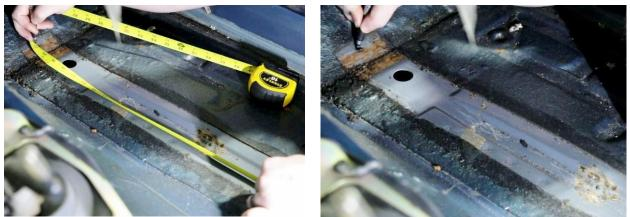
Figure 11 - Mark Front of Cut Area
