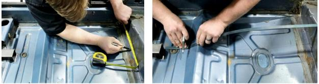
Figure 23 – Mark Outboard Cut Line
