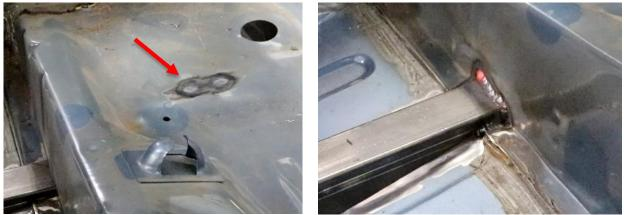
Figure 56 - Weld Seat Riser to Connector
