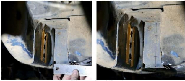
Figure 31 - Locate Plug Weld Holes
