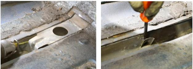
Figure 17 – Remove Floor Pan Bracket
