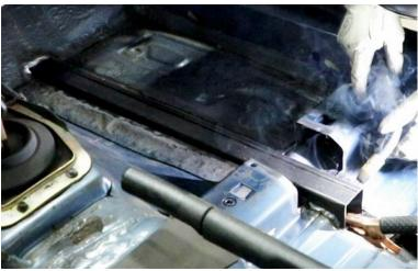
Figure 43 - Weld Sides of Connector
