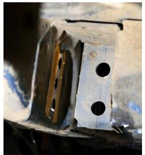
Figure 32 - Drill Plug Weld Holes
