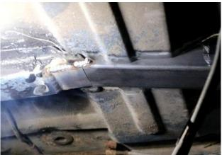
Figure 46 - Weld Sides of Connector
