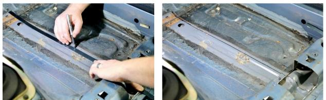
Figure 13 – Mark Outboard Cut Line
