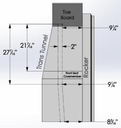
Figure 10 - Floor Cut Lines
