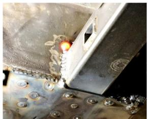
Figure 51 - Weld Rear Connector
