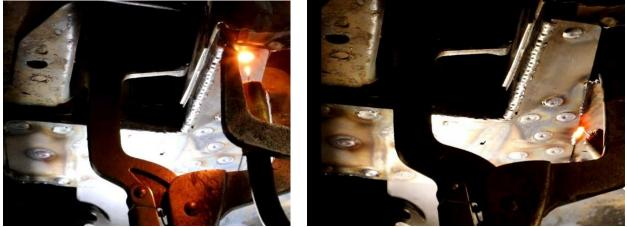
Figure 50 – Plug Weld Torque Box
