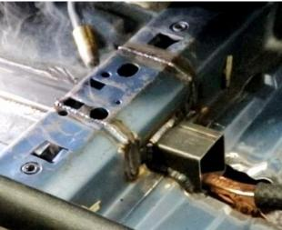
Figure 44 – Weld Seat Riser Section
