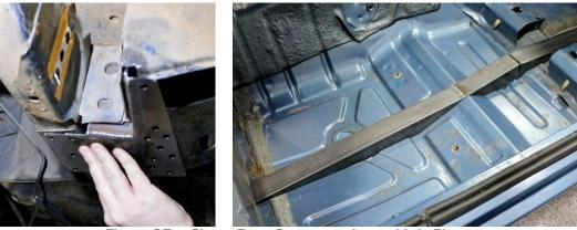
Figure 35 - Clamp Rear Connector Assembly in Place
