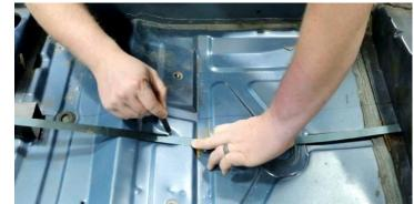
Figure 24 - Mark Inboard Cut Line
