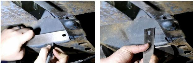
Figure 26 - Locate Lower Link Pocket
