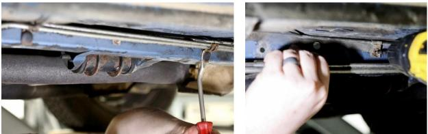
Figure 2 – Remove Fuel & Brake Line Clips
