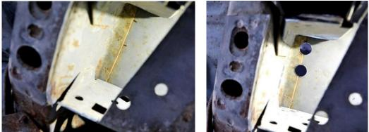
Figure 34 - Drill Plug Weld Holes
