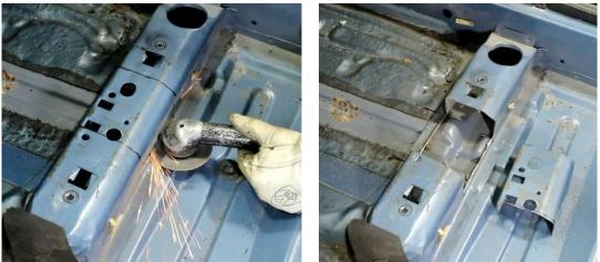
Figure 9 – Remove Seat Riser Section
