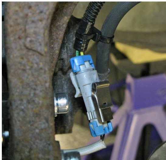
Figure 6 - Connect ABS Sensor
