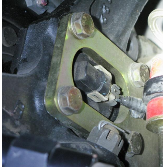
Figure 1 - Unplug ABS Sensor
