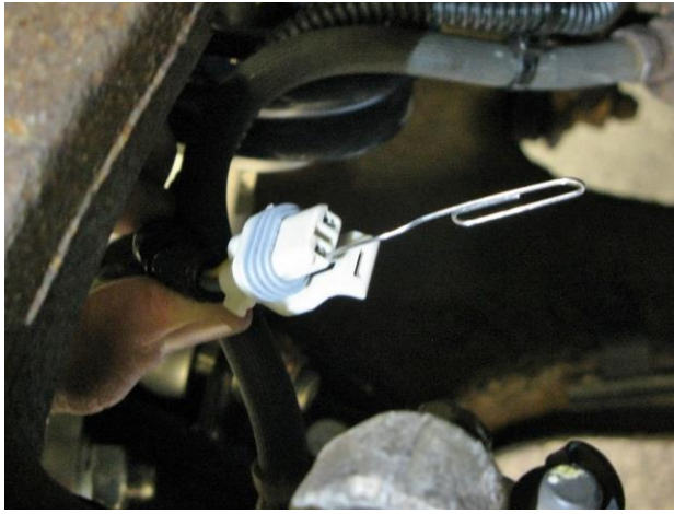
Figure 4 - Remove ABS Terminals
