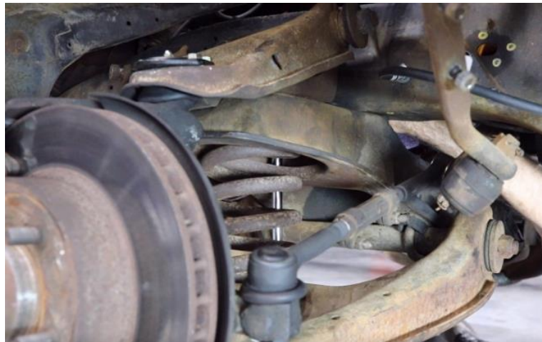
Figure 14 - Remove Cradle Hardware
