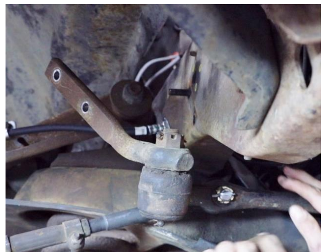
Figure 6 - Remove Idler Arm
