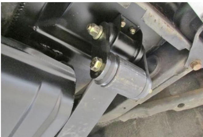
Figure 19 - Install Rear of Leaf Spring
