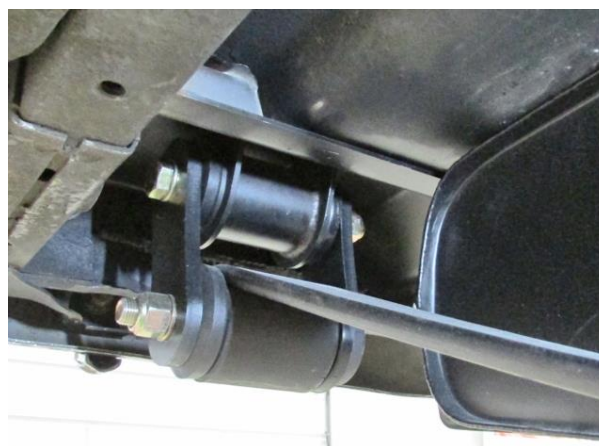
Figure 19 - Install Rear of Leaf Spring
