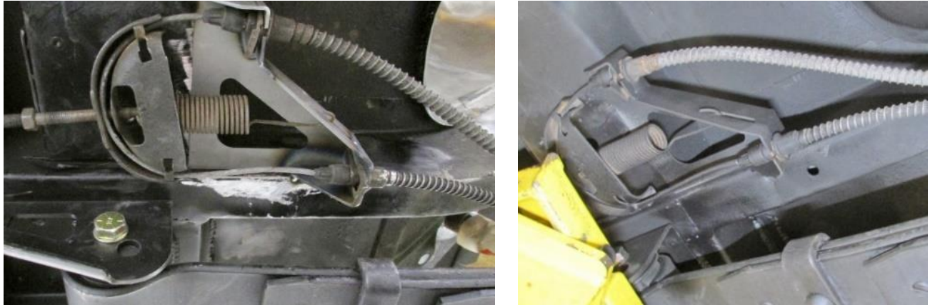
Figure 23 – Install E-Brake Cable Bracket
