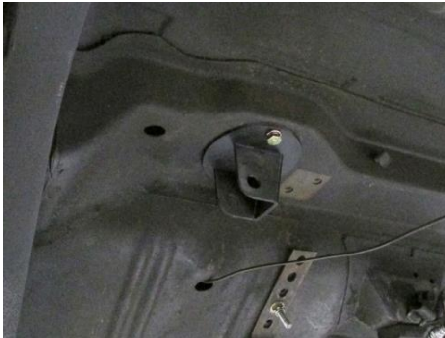
Figure 17 - Install Shock Assembly (Driver Side)
