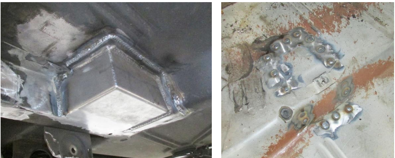
Figure 9 - Weld Torque Boxes
