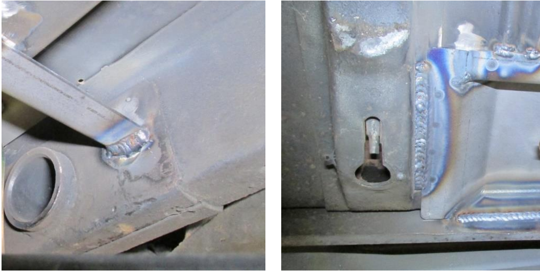
Figure 13 – Weld Mount to Vehicle
