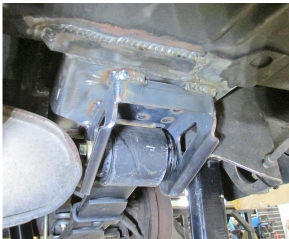
Figure 18 - Install Front of Leaf Spring
