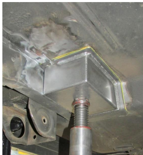
Figure 6 – Mark Floor Pan for Plug Welds
