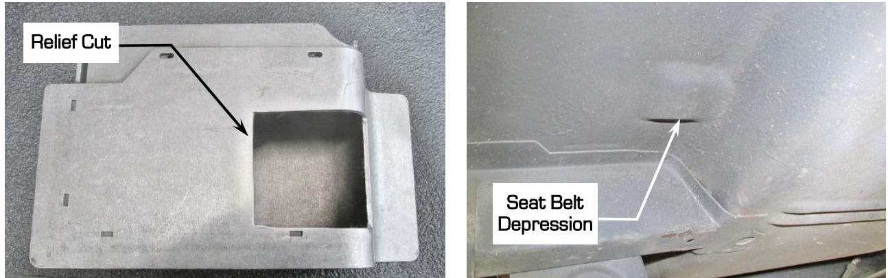
Figure 7 - Relief Cut Torque Boxes
