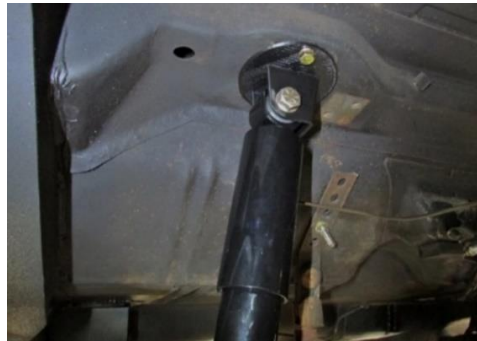
Figure 21 – Install Shocks to Upper Shock Mounts
