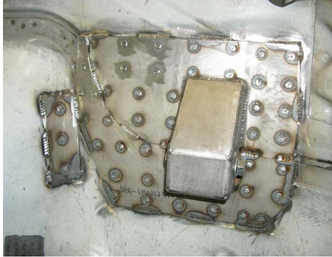
Figure 11 - Stitch Weld Tunnel Doubler
