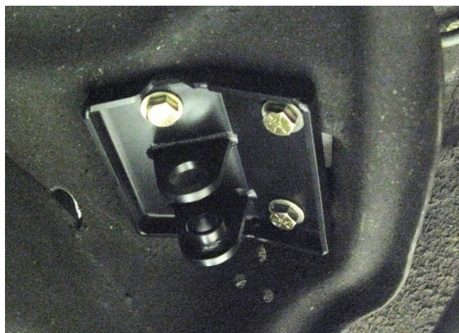
Figure 2 - Installed Upper Coilover Bracket
