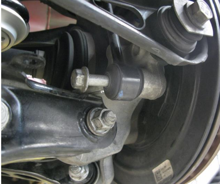
Figure 16 - Re-attach Sway Bar End Links
