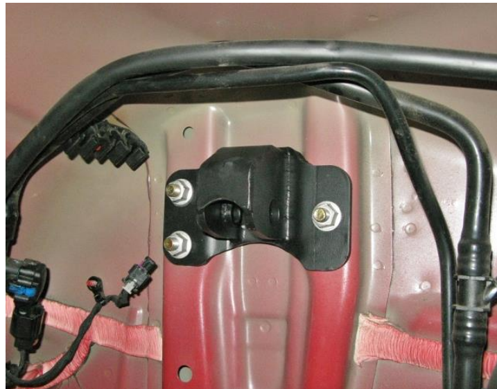
Figure 10 - Install Upper Shock Mount
