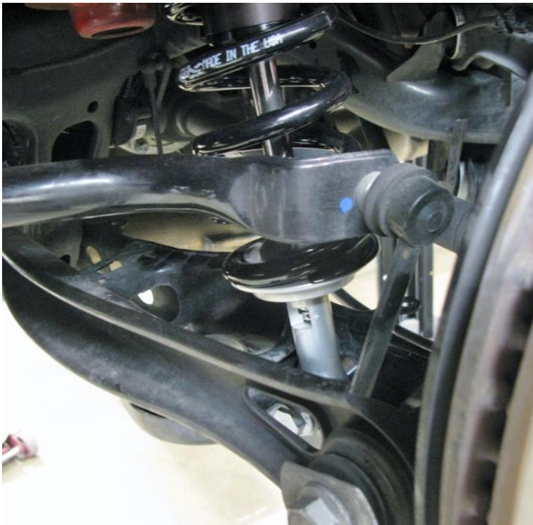
Figure 17 - Final Coilover Shock Assembly
