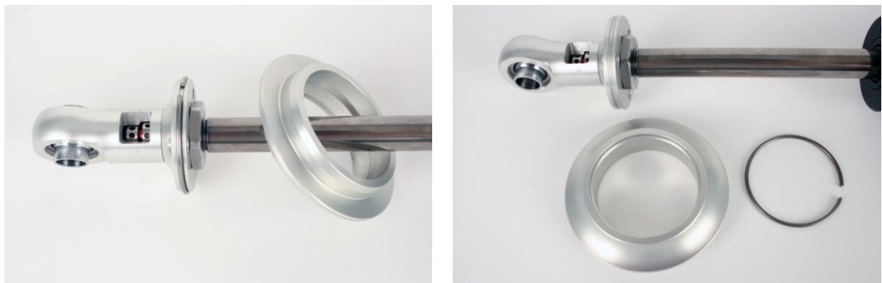
Figure 12 - Remove Spring Seat & Retaining Ring
