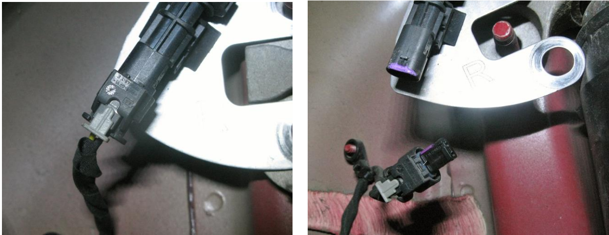
Figure 7 – Disconnect Magnetic Ride Control
