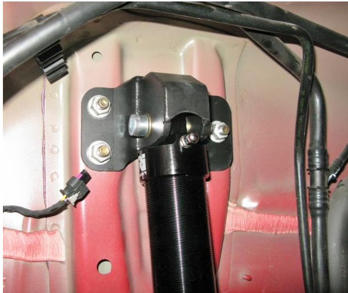
Figure 11 - Install Coilover Shock
