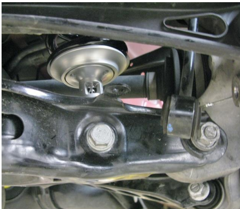
Figure 15 - Re-attach Lower Control Arm & Trailing Link
