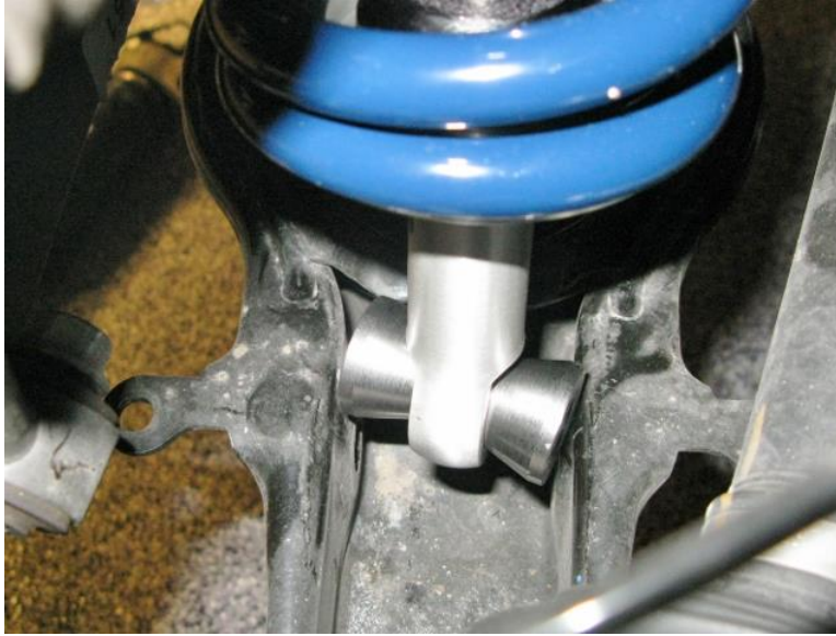
Figure 14 - Install Tapered Spacers
