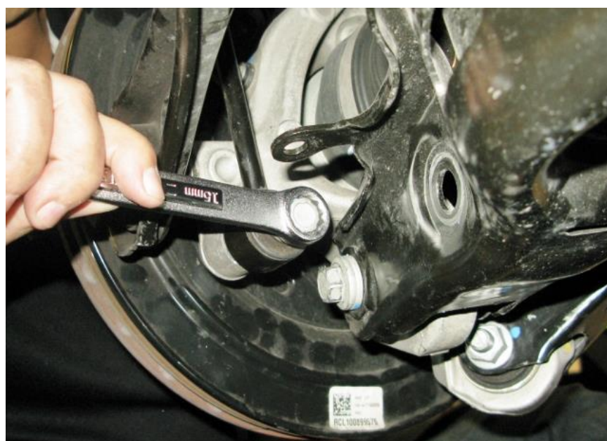
Figure 4 - Disconnect Sway Bar End Links
