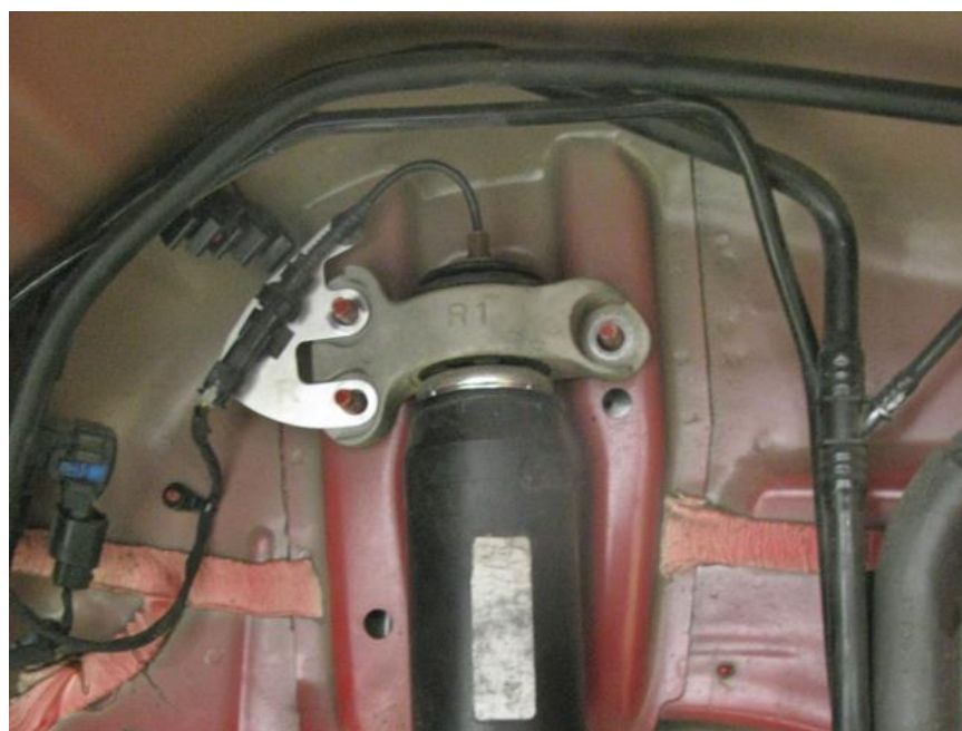
Figure 6 – Remove Upper Shock Mount Nuts
