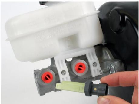
Figure 4 – Removing Sensor
