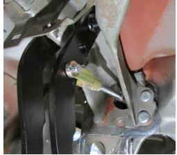
Figure 2b – Install Clevis Pin
