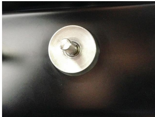
Figure 7 - Thread Bezel onto Switch
