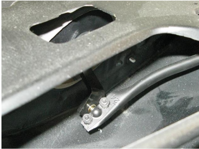
Figure 3 - Attach Pitman Arm to Wiper Linkage
