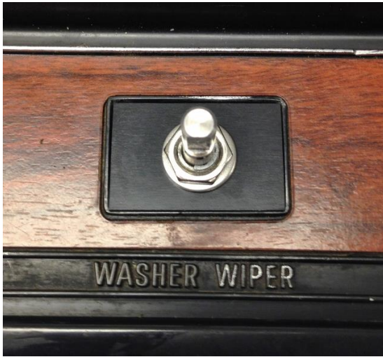
Figure 11 - 1969 Camaro Switch/Knob Installation
