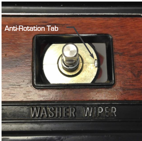
Figure 10 - Install Wiper Switch & Alignment Plate
