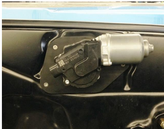
Figure 2 – Attach Wiper Motor to Firewall
