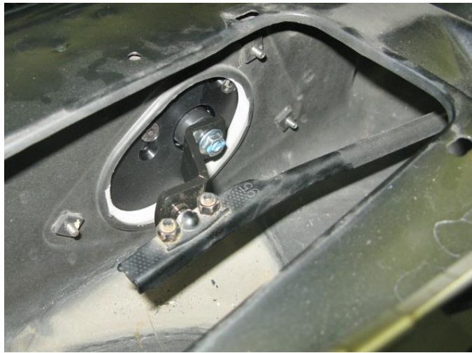
Figure 3 – Attach Pitman Arm to Wiper Linkage
