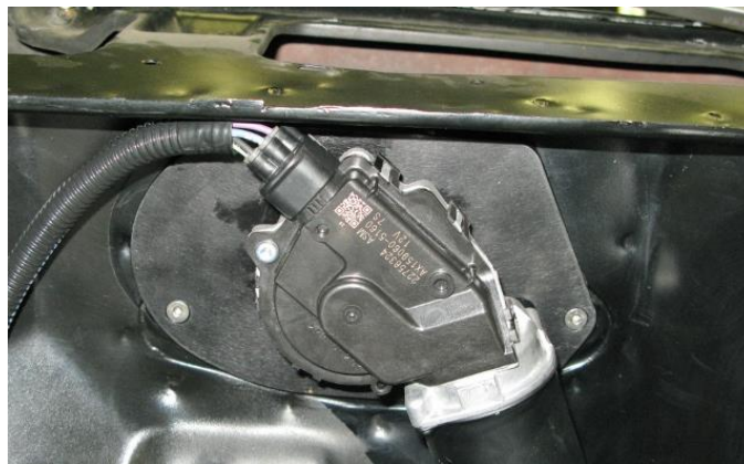
Figure 7 - Install Wiper Motor Connector (P/N: 121406 Shown)
