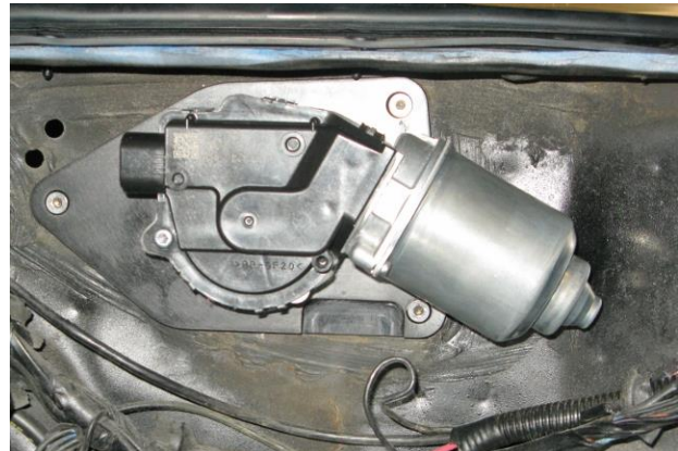
Figure 3 - Wiper Motor Orientation (P/N: 121408 Shown)
