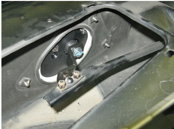
Figure 4 – Attach Pitman Arm to Wiper Linkage
