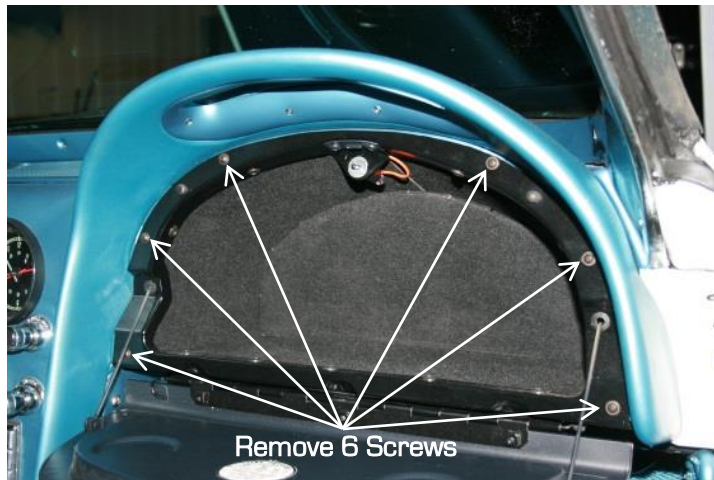
Figure 3 - Remove 6 Mounting Screws
