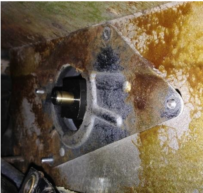
Figure 12 - Mount the Wiper Motor
