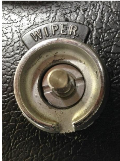
Figure 19 – Install Switch Nut
