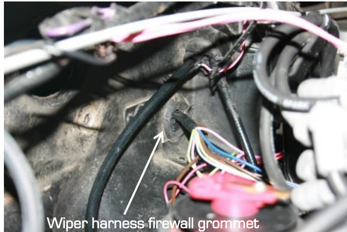
Figure 8 - Remove Firewall Grommet
