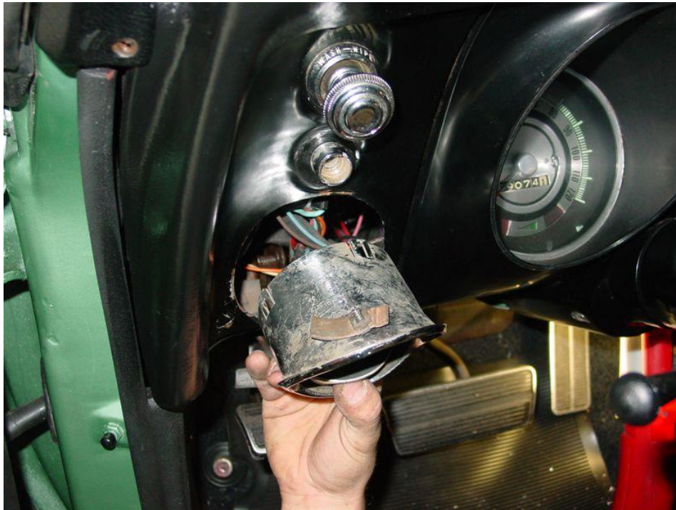
Figure 4 - Removing the Astro Vent
