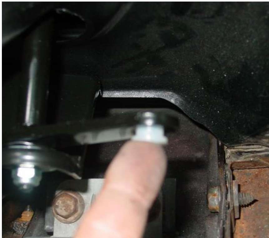
Figure 13 - Installing Bushing in Pitman Arm
