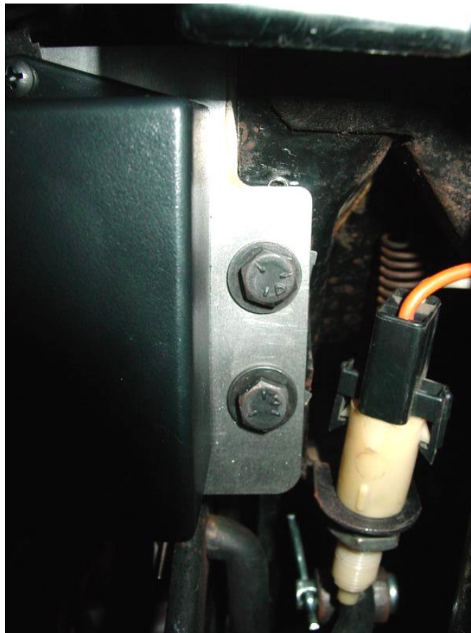
Figure 3 - Module Mounted in Place
