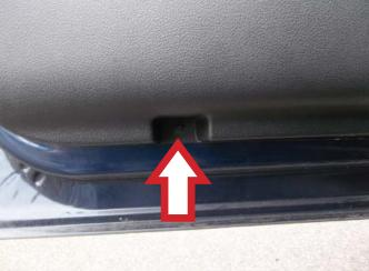
**STEP 4:** Using a trim panel removal tool, release the speaker grille assembly.
