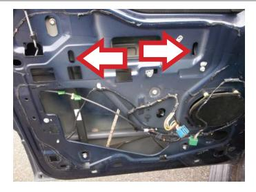
**STEP 5:** Manually slide the window glass to align the screws attaching the window glass to the window regulator.
