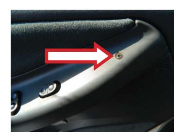
**STEP 13:** Using a Phillips head screwdriver, install the interior door handle bezel assembly.
