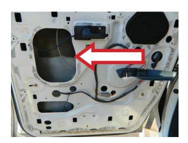
**STEP 2:** Using a 10mm socket and ratchet assembly, attach the upper part of the window regulator.
