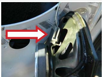
**STEP 8:** Remove the water vapor barrier.
