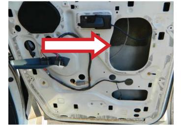
**STEP 2:** Using a 10mm socket and ratchet assembly, attach the upper part of the window regulator.
