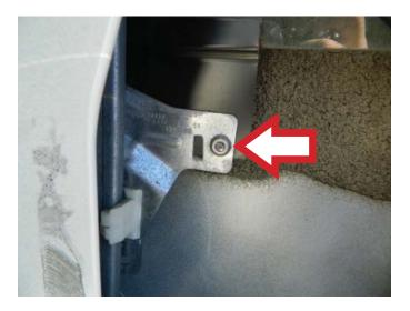
**STEP 6:** Manually slide the door glass into position and attach the door glass using Dorman kit # 702-013.
