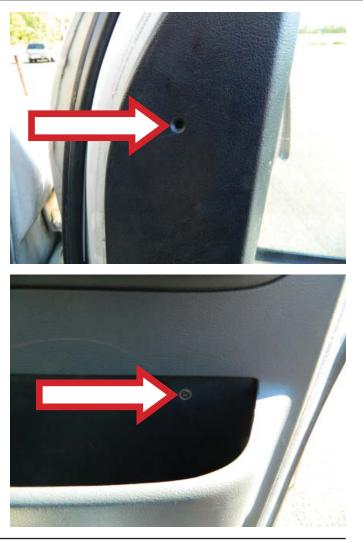
**STEP 15:** Verify that all of the interior door trim panel retaining screws are secure and that the window regulator assembly is operating properly.
