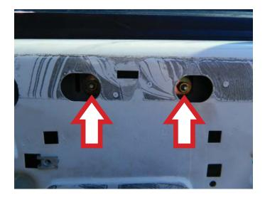
**STEP 13:** Using a 10mm socket and ratchet assembly, remove the two (2) window regulator retaining nuts.
