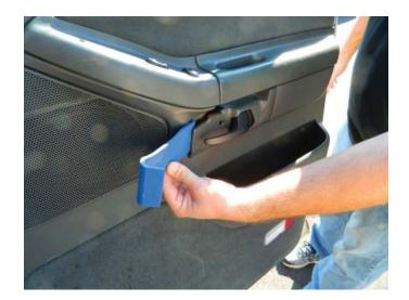
**STEP 4:** To remove the power switch assembly, lift it in an upward motion. Once you have released the power switch assembly, place the switch through the opening of the interior door trim panel.
