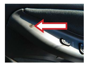
**STEP 13:** Using a Phillips head screwdriver, install the interior door handle bezel assembly.
