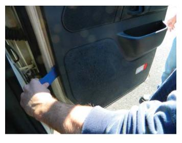
**STEP 3:** Using a trim panel removal tool, remove the interior door handle bezel assembly.
