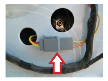
**STEP 11:** Disconnect the window lift motor.
