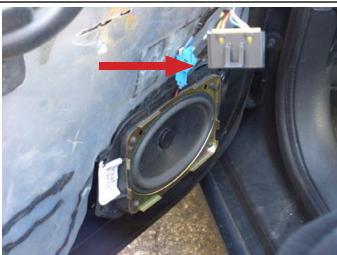
**STEP 6a:** Remove the four (4) screws that hold the door speaker into the door.
