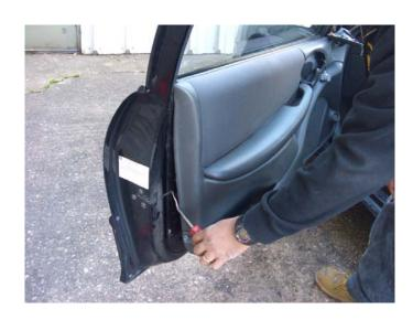
**STEP 4b:** Gently lift in an upward motion to remove the interior panel.
