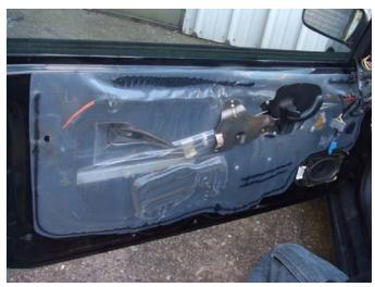
**STEP 6:** Disconnect the electrical connector for the door speaker.
