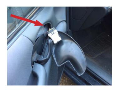
**STEP 3:** Remove mirror bezel assembly and three (3) Phillips head screws holding the door panel on the door.
