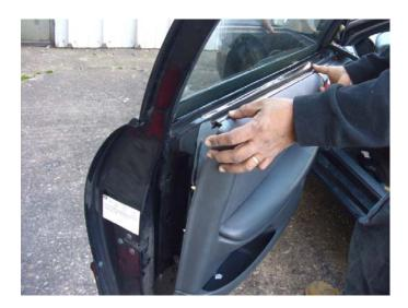
**STEP 10:** Install and connect the door cup assembly.
