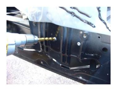
**STEP 11:** Remove the power window regulator from the door.
