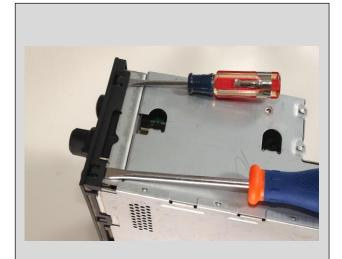
Screwdrivers used to wedge plastic clasps out.
