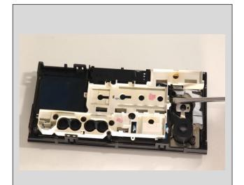
Unclasp plastic tabs using a small thin screwdriver
