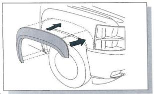
Place the front Fender Flares onto the vehicle and line up the holes on the part with the screw holes on the vehicle.
