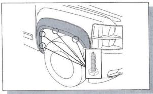
**9.** Re-Install the socket head screws into the fender to secure the Fender Flares. Fit the Fender Flares loosely until the Fender Flares are aligned as desired, when satisfied, tighten the screws fully and ensure extrusion is flush neatly against the body.
