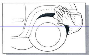
3. Wash the areas of contact on the vehicle and wipe dry both the vehicle and the Fender Flares with a clean cloth. Ensure inside of Fender Flares where extrusion is attached is clean, use alcohol wipe supplied to clean surface.
