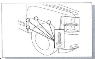
7. Use the original manufacturer's hardware that is in the wheel arch of the vehicle to fit the Fender Flares. Remove the 4x 7mm socket head screws from the fasteners on the vehicle.
