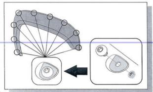
2. Attach 9 bolts to each Fender Flare using a 3/16" Allen key and a 1/2" wrench/socket.
