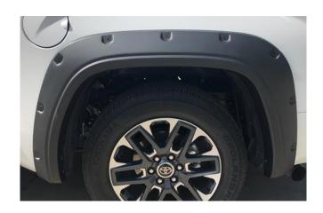
**STEP 19:** If necessary, make minor adjustments to the flare's position to achieve the best fit. Ensure rubber seal is sitting flat against vehicle. When satisfied, fully tighten all screw locations in the above order in which they were just installed. Repeat installation for opposite side.
