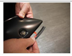
**STEP 2:** Attach the included rubber seal to the Fender Flares. Peel back 2" of the adhesive backing and position on the Fender Flare. Attach the seal to the Fender Flare, peeling back a few inches at a time. Ensure pressure is used to secure rubber seal to Fender Flare edge. Attach rubber seal along the top leading edge of the Fender Flare where it contacts the vehicle body.
