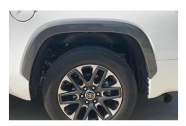
**STEP 14:** Clean the body area where the Fender Flares will contact vehicle surface. Ensure fender surface is dry prior to install.
