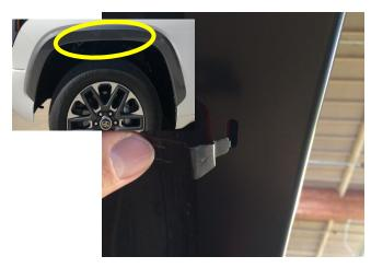
**STEP 9:** Secure attachment clips by sliding clip into Fender Flare slot and using the factory screws that were previously removed in Step: 8 to attach the clips into corresponding existing holes in upper inner splashguard. Do not fully tighten screws at this stage.
