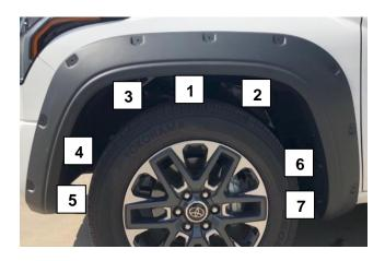
**STEP 10:** Begin to loosely install factory screws that were removed in prior Steps: 7 & 8 into slotted hole locations. Once all factory screws have been reinstalled, apply pressure and begin to tighten in the order shown above.
