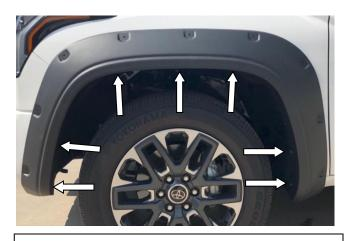
**STEP 6:** Hold Fender Flare on the vehicle in the position of best fit. Note where above marked slots in the Fender Flare, align with the existing mounting holes on the vehicle. Remove the Fender Flare.
