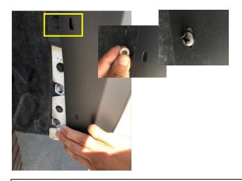
**STEP 17:** POSITION (A2) - Ready the spacers (and long screw) to go in behind the Fender Flare to fill the gap between the flare and the vehicle.
