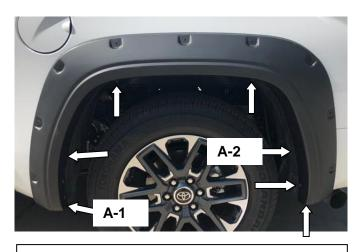
**STEP 15:** Hold Fender Flare on the vehicle in the position of best fit. Note where all the slots in the Fender Flare align with existing mounting holes on the vehicle. Again, make note of position (A-2) as it will require hardware in the kit supplied. All remaining positions will re-use factory screws and plugs.
