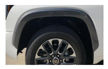
**STEP 5:** Clean the body areas where the Fender Flares will make contact with the vehicle surface. Ensure fenders are dry prior to install. Turn tires facing outward to provide additional room and ease hardware installation per side.
