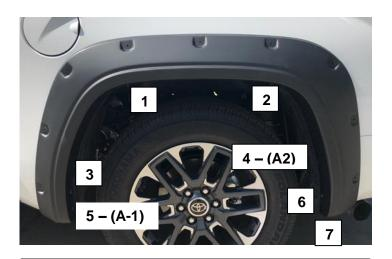
**STEP 16:** Begin to loosely install factory screws that were removed in prior Steps: 12 & 13 into into the corresponding factory attachment points. Once all factory screws have been re-installed, begin to fasten in the order shown above. Do not fully tighten screws at this time.
