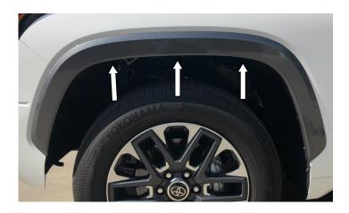
**STEP 8:** Locate and remove the (3) factory screw locations in the upper wheel well. Retain for later re-install.
