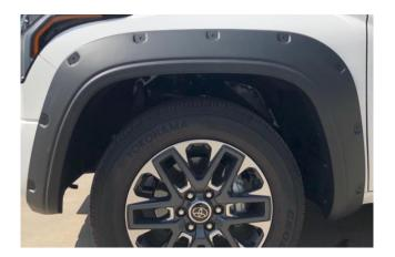
**STEP 11:** If necessary, make minor adjustments to the flare's position to achieve the best fit. Ensure rubber seal is sitting flat against vehicle. When satisfied fully tighten all screw locations, in the above order in which they were just installed. Repeat installation for opposite side.
