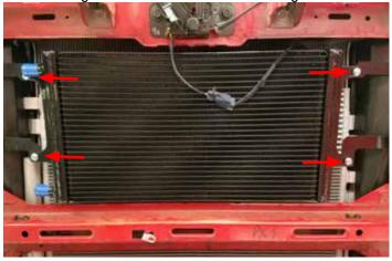
26. Pass hoses #3 and #4 through the new holes in the plastic cowl and Install the hoses onto the LTR using the clamps provided in bag #2. TIP: It's easier to insert the hose from the front of the vehicle. NOTE: Install the supplied 4" pieces of convolute over the LTR hoses to help protect them from chafing.
