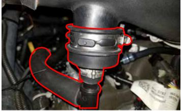
70. Connect the PCV line to the fitting on the intake tube.
