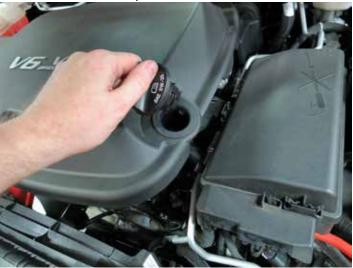
36. Disconnect the intake tube from the throttle body and lift the engine cover up. Disconnect the PCV hose from under the front right of the cover. The cover should be free now. Replace oil cap when finished.
