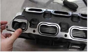
53. Remove the intake port covering. Clean the sealing surface and check for any stubborn dirt or debris before proceeding.
