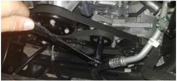
47. Disconnect the vacuum hose as pictured. Remove the bolts in the following picture and set aside. The bolts will be reused on the new bracket. The 13mm bolt has a nut on the opposite side. Be sure to recover this nut since it will be reused. Unplug and remove the vacuum assist pump and bracket from the front of the block, then remove pump from the OEM bracket.
