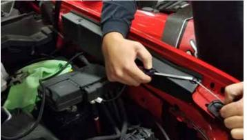
75. Remove the fender attachment bolt and secure the ground to the Water Pump Harness as pictured.
