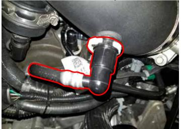
71. Unplug the MAF connector & attach the TMAP harness to the MAF. Reconnect the MAF sensor plug into the TMAP harness. Then connect the last plug into the TMAP extension located on the intake that was installed earlier.
