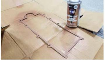
57. Place the gasket on the intake manifold base. Be sure to align the gasket with the holes to ensure a perfect seal.
