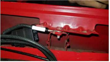
76. As you reinstall the panel, secure the relay by inserting the push-pin through the panel and then through the relay mounting tab.
