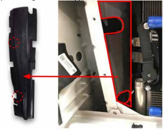
24. Reinstall the plastic cowl and install the LTR brackets (Shown in red) by reusing the bolts that were removed when uninstalling the shutters assembly. **NOTE:** PEM nuts face towards rear of vehicle.
