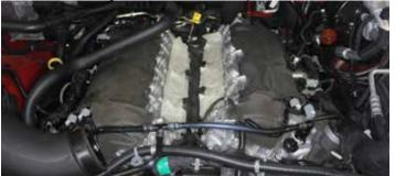
44. Using a 13mm socket, remove the front engine cover bracket. Renstall the original bolt in the passenger side.
