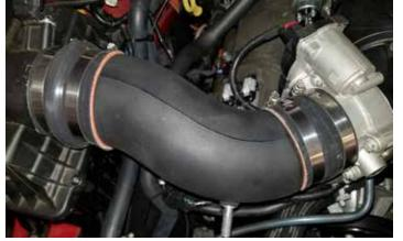
69. Reconnect the factory crank case ventilation hose to the bottom of the new intake tube.
