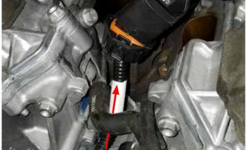
55. From bag #3, install the (7) M8 x 65mm bolts, and the (1) M8 x 30mm intake bolt in the back. Use the following sequence to torque the bolts to 18 ft/lbs. (#8 bolt is the short bolt) using blue Loctite.
