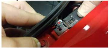
77. Replace the grill shutters by unbolting the LTR backets to the core support <u>on one side only</u>. Install the shutters back on and replace the bolts that were removed on that side. Once the grill shutters are tight on the one side, do the same for the other side. Doing this helps keep the LTR in place while you install the bolts. This makes it a lot easier to reinstall.
