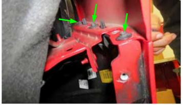
17. Remove (2) 10mm bolts from the center of the grill. NOTE: They are deep inside and can be hard to see. Do this for each side. **NOTE:** ZR2 models have (4) 10mm bolts.
