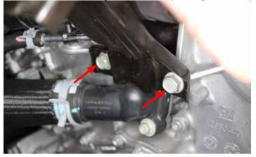
45. Remove the factory timing cover bolts (pictured) and install the wire harness support bracket using the original bolts.
