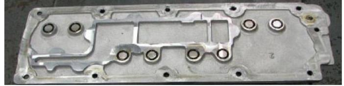
34. Apply anti-seize to the tapered surface beneath the heads of the countersunk bolts supplied in Bag #3. Install the bolts, along with the valley plate and the stock perimeter gasket. Use a 5mm hex socket tighten the bolts from the center out and in a criss cross pattern to 18 ft-lbs.
