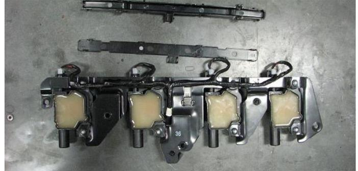
50. Tuck any loose wiring under each coil bracket then use a 10mm socket and the ten stock bolts to install the coil brackets on to each valve cover.
