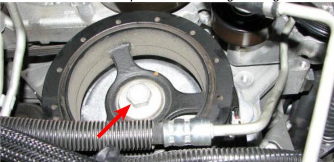
16. Install the drill guide and the M16 x 120mm guide bolt supplied in Bag #4 onto the end of the crankshaft.
