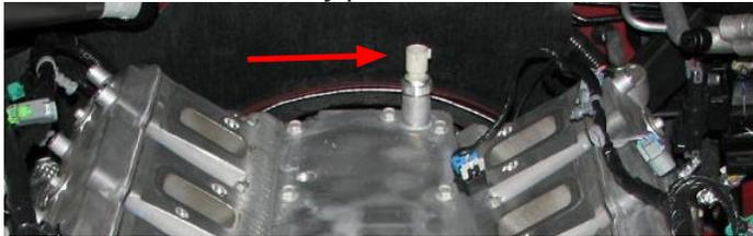
32. Clear the engine valley of all debris, remove the 11 bolts with a 13mm socket, then remove the valley tray.
