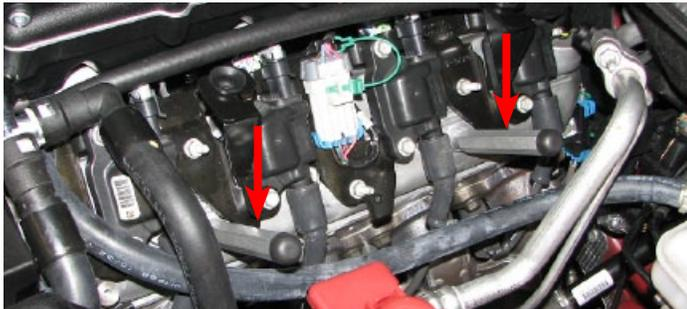
115. Use a 10mm deep socket to install the supplied ball studs into the new coil covers.
