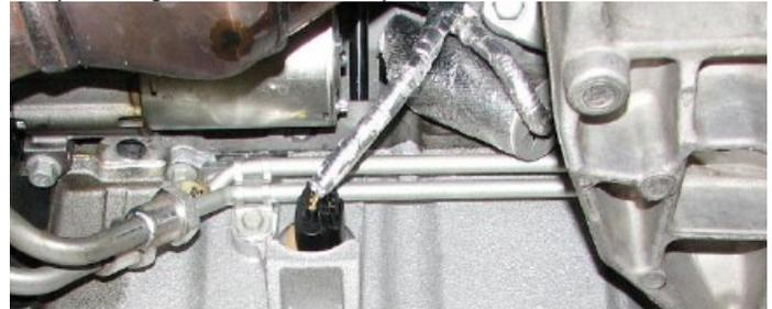
8. Use a 10mm socket to remove the starter support bracket bolt.
