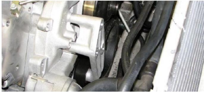
57. Apply blue Loctite to two stock tensioner bolts which were removed during Step 53. Mount the new tensioner bracket onto the water pump using the stock bolts and a 15mm socket. Apply blue Loctite to the M10 X 45mm bolt supplied in Bag #1 and install the bolt to the left provision on the bracket. Torque all three bolts to 37 ft-lbs.
