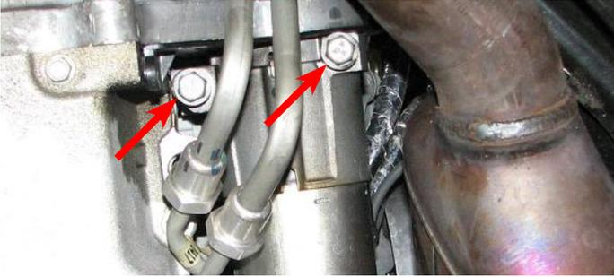
10. Use an 8mm wrench to remove the three bolts retaining the starter heat shield.
