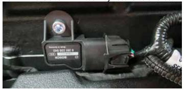
40. Apply O-ring lube to the O-ring on the EVAP solenoid and install onto the supercharger manifold using the factory EVAP solenoid bolt.
