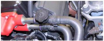
**47. CAMARO ONLY:** Install the driver and passenger side coil covers over the hoses using three (3) M6 x 40mm bolts and one (1) M6 x 35mm bolt from hardare bag 4. Oil fill cap will need to be removed before placing the driver side cover.
