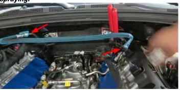
22. Using a pry tool with smooth edges, remove the factory PCV seal from the bottom of the factory supercharger. TIP: It's best to pry the seal on the metal base as to not tear the upper rubber portion. NOTE: In the event this PCV Seal is missing or damaged contact Edelbrock Tech Support @ 800-416-8628 to purchase a replacement seal P/N 51-4301.
