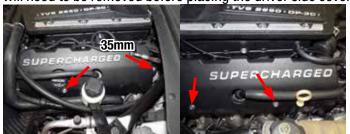
48. Verify no hoses were pinched during installation of the coil covers. Re-position as needed.
