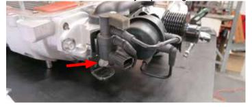
30. Remove the solenoid from the solenoid bracket. Using a Q size drill bit, open up the mounting hole on the solenoid bracket. Deburr the bracket as needed.
