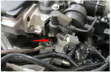
10. Disconnect the EVAP solenoid connector.
