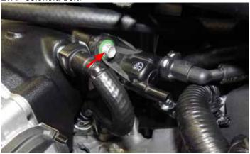
41. Connect the quick connector on the factory brake booster hose to the supercharger.
