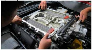
18. Cover the ports with protective tape to keep out debris. Remove the black foam insulator from the valley and set aside.
