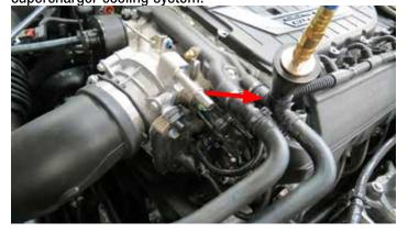
4. Using a small flathead screwdriver, remove the locking clips securing the coolant hoses to the water crossover and remove. Place lines into a small container to prevent coolant leakage.
