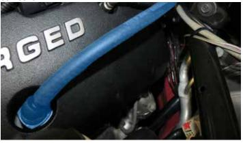
51. Install the supplied bypass hose onto the fitting on the bottom of the actuator then over the cover to the manifold as shown.
