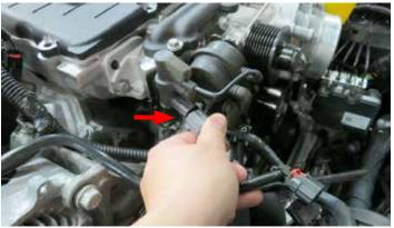
9. Using a panel puller, remove the harness retaining tree clip from the actuator solenoid bracket.
