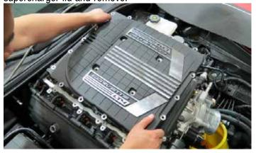
15. Using a 10mm socket, remove ten (10) bolts securing the supercharger manifold to the cylinder heads.
