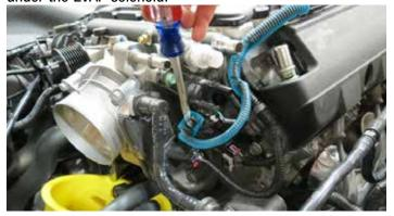
12. Release the blue locking clip on the electronic throttle body connector and remove the connector from the throttle body.
