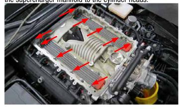
16. Carefully position the supercharger manifold forward to access the TMAP sensor. Disconnect the TMAP sensor connector.
