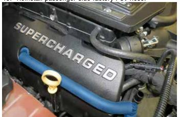
50. Connect driver side pcv hose through the hole in the coil cover.
