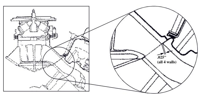
All four walls of manifold port should be .025" less than cylinder head port.
