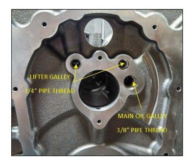
Part # 450000, 450001 Rev. 2/21/18 - NP NOTE: If your engine requires an oil cooler or dry sump set up, you must install a 5/8" core plug to the bottom of the step in the red outlined oil galley located under the oil filter housing. An additional bypass is also required under the oil filter adapter as shown below.
