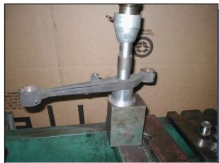
A hydraulic press was used to remove the original bushing, including the outer metal casing the rubber is bonded to. The inside diameter of the control arm is Ø 37mm (1.457"). Go about .050" smaller when pressing out the bushing.
