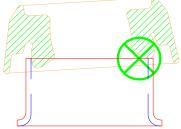
Place the upper vertical bushing #3370 in the metal shell first, this enables you to confirm that the inside edge of the bushing is not pinched at the top of the shell.
