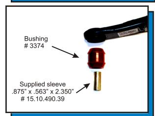
Note: Make sure to thoroughly grease all surfaces of bushing that contact metal.
