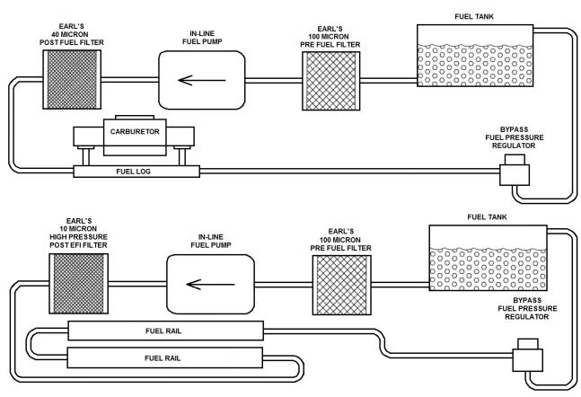
Figure 4b (Both carb & fuel injection applications)
