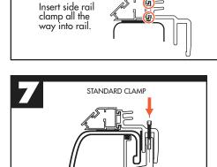
Attach "U" clamp to side rail clamp with allen bolt. Insert side rail clamp
