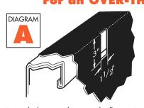
For each clamp mark on your bedliner a  $1-1/2'' \times 3''$  hole as shown above. Remove clamp. Cut holes in bedliner. Reinsert side rail clamp. Return to step 6.
