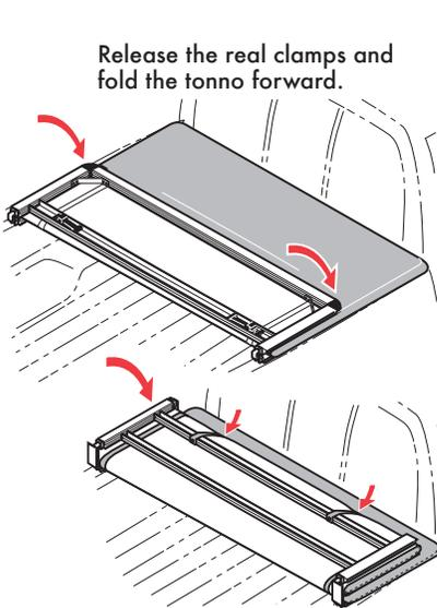
**IMPORTANT:** Before folding the second section of the tonno, rear clamps must be stowed into the rear bow to prevent damage to fabric.
