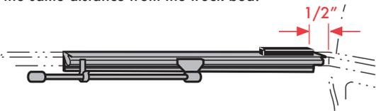
Align the top of the underbody rail flush with the top of the truck bed and secure the clamps as shown.
