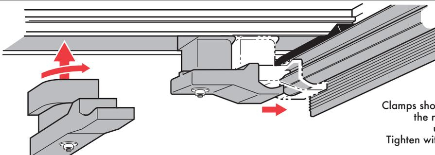
Clamps should be fully secured under the radius section of the underbody rail.
