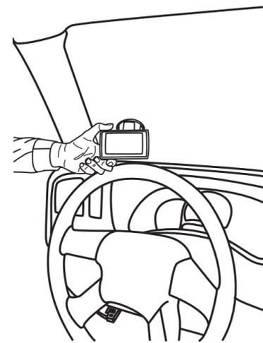
Once you've identified the suction cup position on the windshield, use the supplied alcohol wipe to thoroughly clean the area. After you've wiped the area clean, let it dry for 2-3 minutes.
