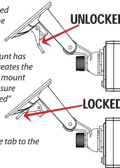
Once you've locked the mount to the windshield, use the adjustment knobs to fine tune the viewing angle and height of the the CTS/CS device.
