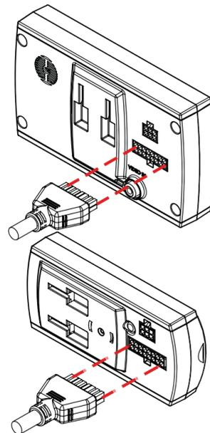
Next, insert the connector on the end of the OBDII cable into the 16-pin connector on the back of the device (this is easier if done prior to mounting the device on the window). The connector only fits one way so be sure that the locking tab is on the bottom.
