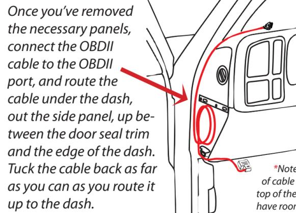
Once you've removed the necessary panels, connect the OBDII cable to the OBDII port, and route the cable under the dash, out the side panel, up between the door seal trim and the edge of the dash. Tuck the cable back as far as you can as you route it up to the dash.
