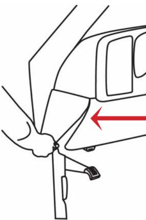
Remove the panel on the side of the dashboard to provide access to route the OBDII cable from the OBDII port up to the top of the dash.
