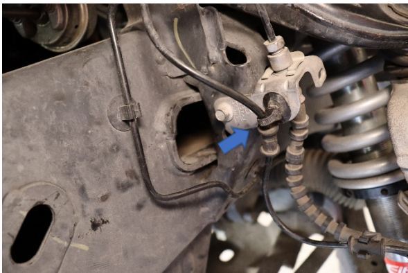
Step 16. Reattach the wheel speed sensor to the upper brake hose bracket.
