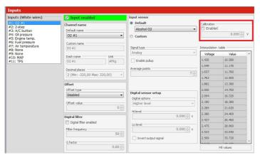
For NTK sensors, free air voltage is around 3.000V. For Bosch sensors, free air voltage is around 2,700V.
