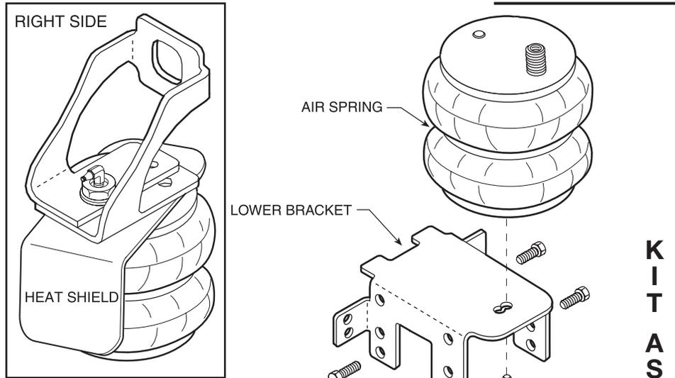
**NOTE:** This diagram is of the left side of the truck. Reverse any orientations when assembling and installing the right side of the vehicle.
