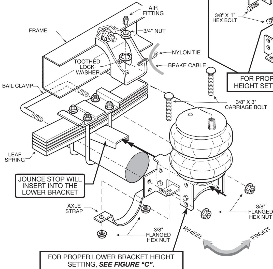
**Note:** This diagram is of the left side of the truck. Reverse any orientations when assembling and installing the right side of the vehicle.
